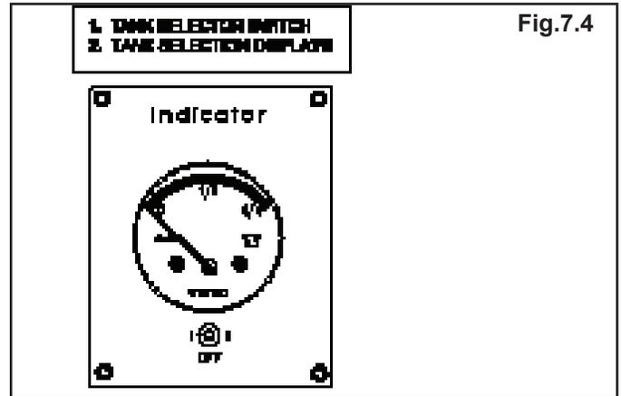
The power switch turns the monitor on, then select the tank you want to monitor. The gauge will show the amount remaining in the tank(s).
