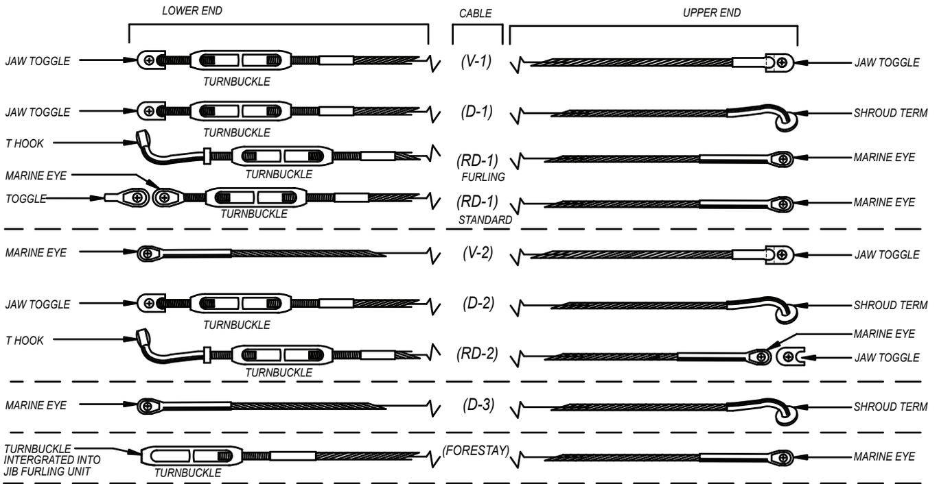
Figure 12.12 Standing Rigging Details
