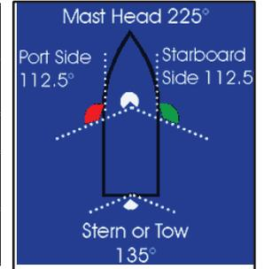
The arc of the lights and color allows you to determine the direction a vessel is moving. How good are your lights? You should test them to see how visible you might be at night. Whether on a trailer or at the marina, switch on your lights and see how well they can be seen. Walk away from the boat or row away, if you are at anchor or at a mooring, and see how visible the lights are as you move further away. How easy are they to see against the background of lights on shore?
