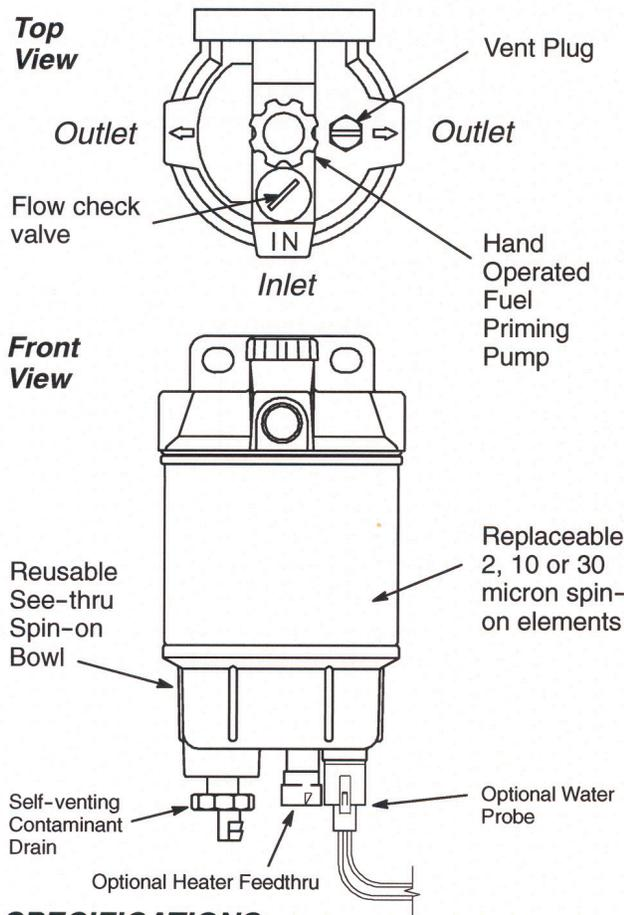
Racor's 215R, 230R, and 245R Fuel Filter/Water Separators are specifically designed to handle today's tough diesel filtration problems. These units feature a standard in-head fuel priming pump and are different from one another only in flow capacity and element size.
