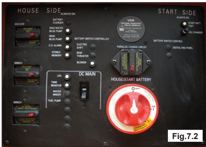
The battery switch panel houses the breakers for some of the main components in your DC system. The breaker controls are marked at the switch panel, and control systems or components on your boat that require a connection that remains energized even through the Main Panel may be de-energized.
